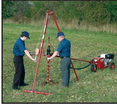
When deeper holes are required, the tripod kit provides controlled drilling and easy auger removal. Using a 4" auger and extensions, holes up to 35' can be easily drilled. Designed for soil sampling and geophysical work, the Tripod Kit features fast set-up, a hand winch, and works with the 11 horsepower Hydraulic Earth Drill and one or two-man handles.
