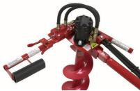
The one-man handle is used for ordinary drilling tasks. The 150 RPM motor generates 225 ft. lbs. of torque to drive augers up to 9" in diameter. An optional 220 RPM motor is available when higher speeds are desired.
