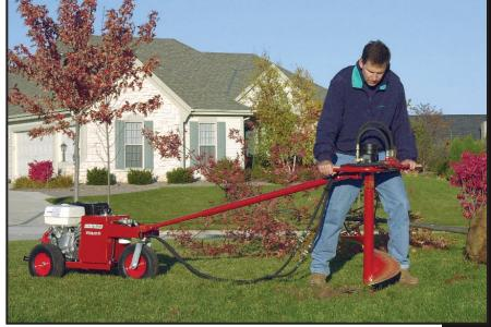
Even with all this power, most hole drilling remains a one-man operation, thanks to our patented torque tube. The torque tube eliminates the kickback found on competitive earth drills, making one-man drilling safe, fast and productive. Convenient front and rear handles make it easy to load the hydraulic earth drill into and out of your truck.
