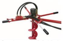
Choose the two-man handle for drilling larger diameter (10"-16") or extra deep holes. It features a standard 150 RPM motor. Faster (220 RPM) and slower (125 RPM) motors are available as options when hole digging requires greater drilling speed or added torque.
