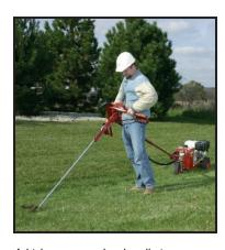
A high-torque anchor handle is designed for anchoring mobile homes or light utility work. At 60 RPM, the standard anchor handle generates 360 ft. lbs. of torque. Optional 125 and 150 RPM motors are also available and are ideally suited for driving bucket augers when performing foundation repair work.
