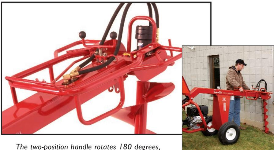
The two-position handle rotates 180 degrees, allowing you to drill right next to buildings, walls, or other obstructions. An infinitely variable 20° auger tilt provides vertical drilling in uneven terrain.
