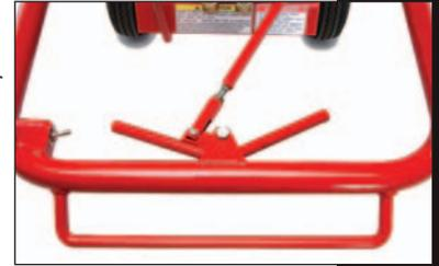
An auger lock makes it easy to maneuver the HYD-TBI IH around the job site.
