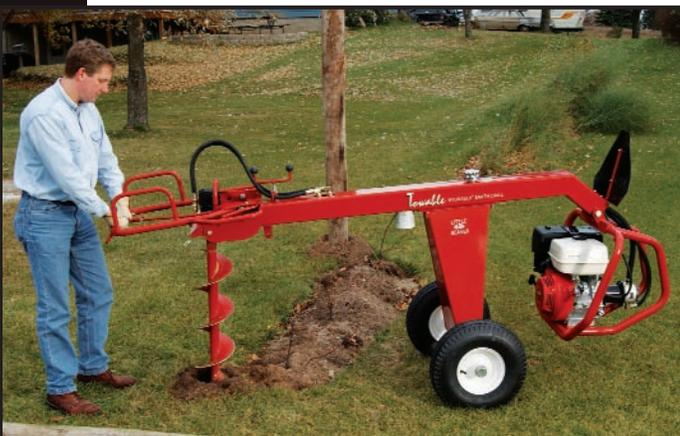
*Pneumatic wheels let you easily move the HYD-TB11H without damaging turf. The machine is incredibly well balanced, requiring less than 20 pounds of force to pivot to the digging position.*
