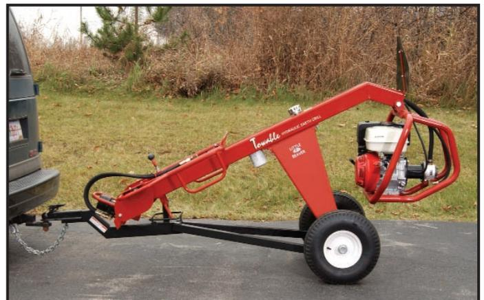
*The towable design saves valuable truck or trailer space. Simply install the standard, removable tow bar, attach to your 2" ball, and connect the safety chains.*
