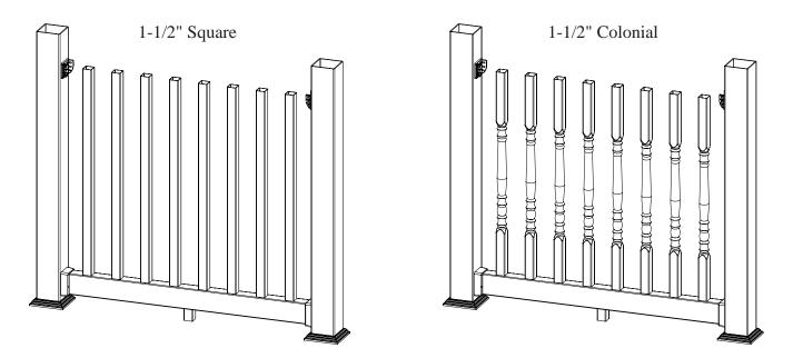
**Step 5 - Insert the balusters.** Having secured the bottom rail into place, insert the balusters into the bottom rail. If the 1-1/2" colonial balusters are being used make sure the balusters are inserted so the baluster tapers are uniformly installed.
