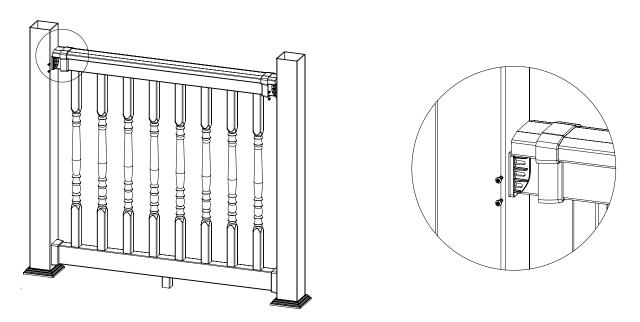
**Step 7 - Secure the top rail.** Position the top rail over the exposed ends of the balusters so that it is positioned on the resting flange of the installed nylon post brackets. Attach the top rail to the nylon post brackets by using the (4) #10 x 1" pan-head screws. Fasten two screws into each side of the nylon post bracket using the top and bottom slots of the nylon post brackets. Snap the alzar bracket covers positioned in Step 6 onto the nylon post brackets.
