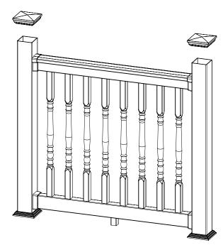
**Step 8 - Finish the section.** Secure the 4" x 4" post caps onto the post tops by applying PVC adhesive to the internal surfaces of the post caps. Set the caps onto the post tops. Wipe off any excess adhesive.
