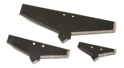
These blades mount to the bottom of standard augers, replacing both the standard point and side cutting blade. Grade 5 mounting bolts and locknuts are included with the 4" to 14" carbide blades.
