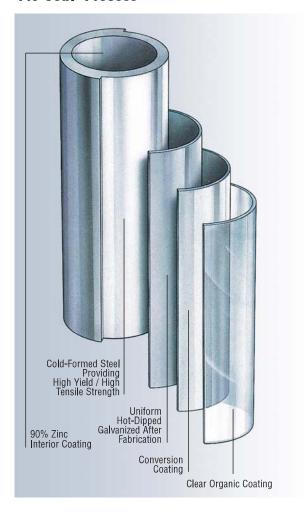
Allied Tube & Conduit, with an engineering breakthrough in pipe manufacturing and corrosion resistant coating, has developed the most specified and the most requested framework in the fencing industry.
