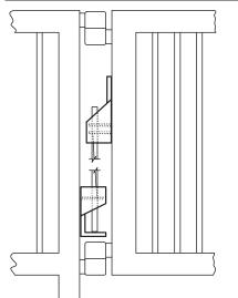
up to six torsion rods can be used for heavier gates
