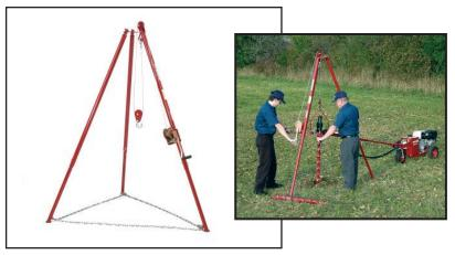
When deeper holes are required, the tripod kit provides controlled drilling and easy auger removal. Using a 4" auger and extensions, holes up to 35' can be easily drilled. Designed for soil sampling and geophysical work, the Tripod Kit features fast set-up, a hand winch, and works with the 11 horsepower Hydraulic Earth Drill and one or two-man handles.
