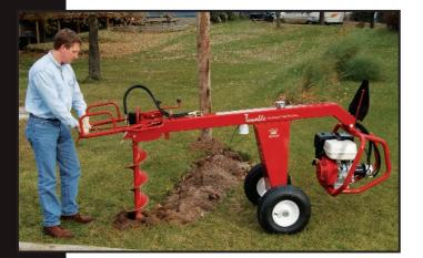
Pneumatic wheels let you easily move the HYD-TBIIH without damaging turf. The machine is incredibly well balanced, requiring less than 20 pounds of force to pivot to the digging position.
