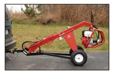
The towable design saves valuable truck or trailer space. Simply install the standard, removable tow bar, attach to your 2" ball, and connect the safety chains.
