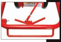
An auger lock makes it easy to maneuver the HYD-TB11H around the job site.
