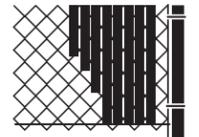
There is no need to kneel down! Simply insert the slats vertically from top to bottom, keeping the locking holes on top.
