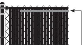
Thread the flexible locking channel horizontally through the notched holes in the slats.
